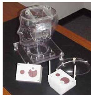
Figure 1 (left): IROC's head and neck phantom
